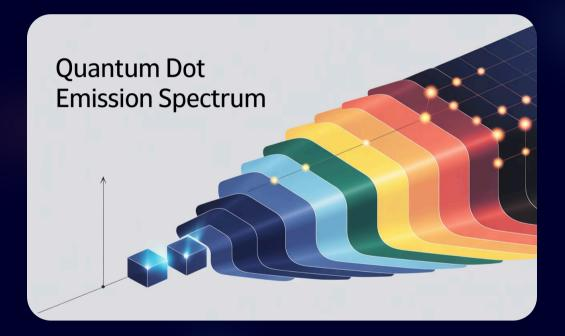
Illustration: Smaller quantum dots (left) confine electrons more tightly, resulting in higher energy (blue) emission, while larger dots (right) produce lower energy (red) emission.
